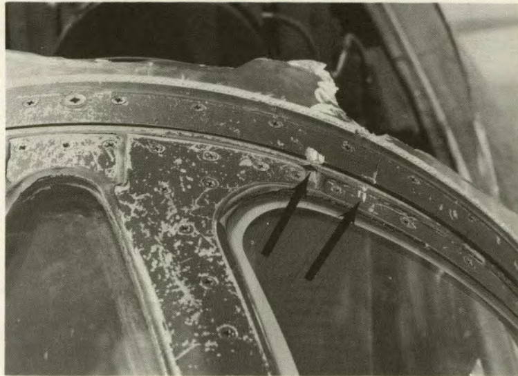
Ricochet impact on canopy bow
